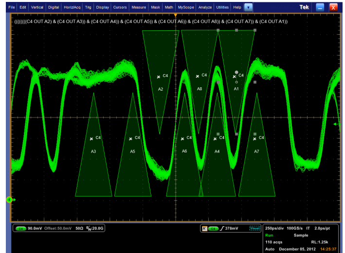
Customized serial triggering. Visual Trigger set to find a serial data pattern of 1101 0101.
